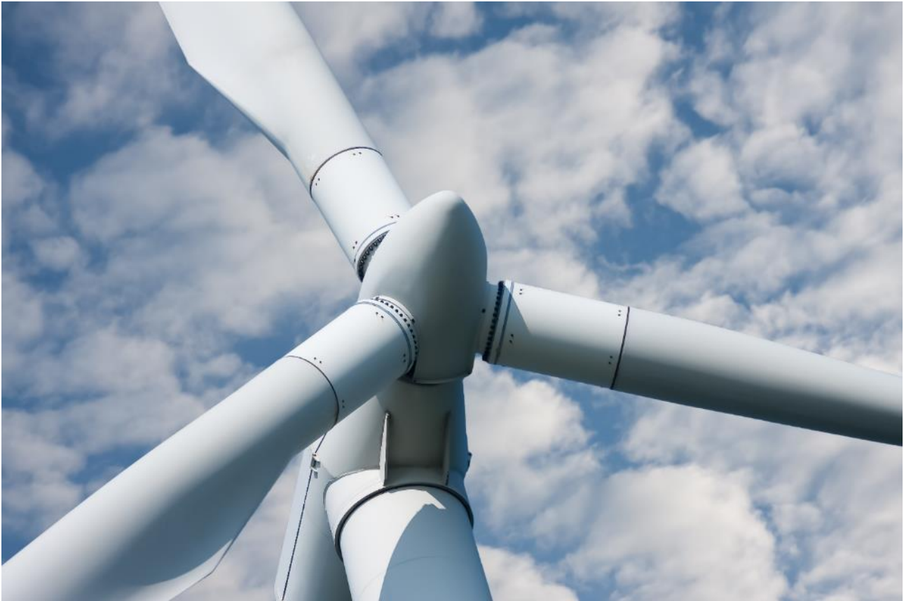
Large wind turbine – only possible with composite materials
