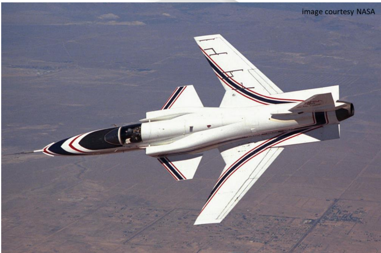
Forward swept wing – only possible with composite materials
